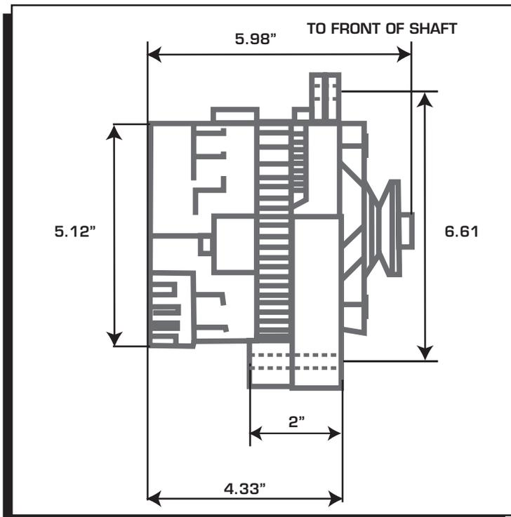
**Figure 2 Alternator Dimensions.**
