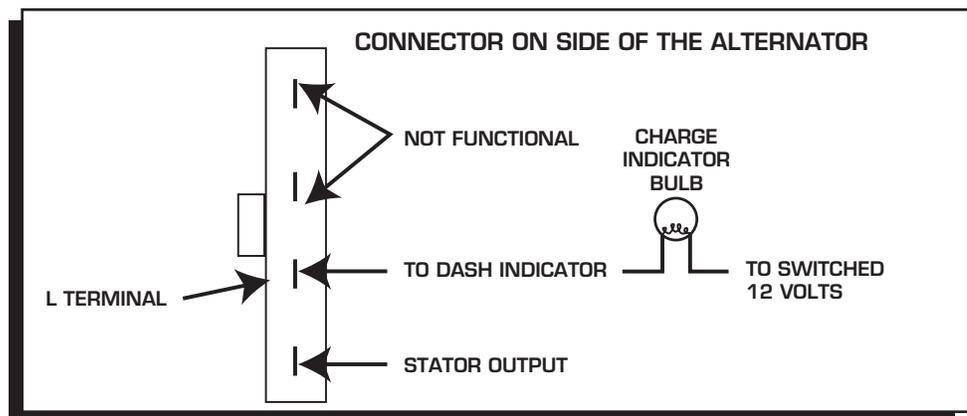
Figure 5 Connecting the OE Charge Lamp Indicator.
