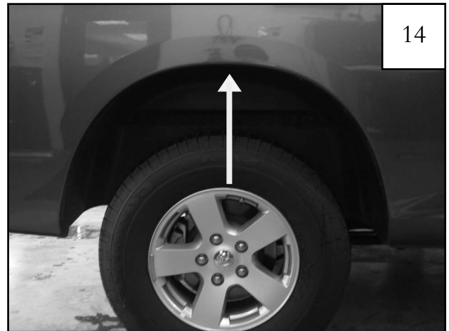
Install Clip (CL1-0022) in this location. See Step 15.
