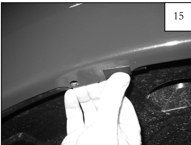
Install plastic tab over existing factory hole.
